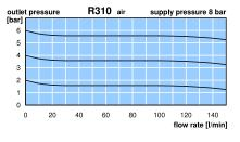
\*1 for compressed air: 8 bar supply pressure, 4 bar outlet pressure and 1 bar pressure drop \*2 01 = 0...1 bar, 04 = 0...4 bar, 10 = 0...10 bar, 16 = 0...16 bar
